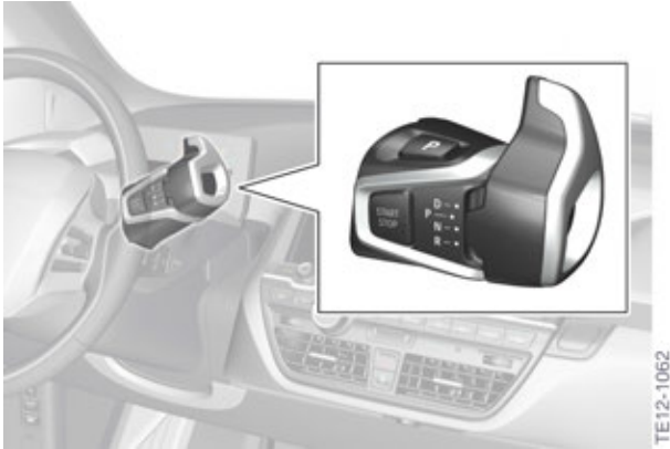
Gear selector switch
